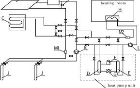
A-solar collector B-expansion valve C-storage tank D-evaporator E-condenser F-compressor G-expansion valve H-terminal unit(fan coil) J-soil heat exchanger K-circulation pump1 L-circulation pump2 M1 \ M2-flow meter N-magnetic valve
