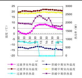
Fig.5 Curve of temperature and supplied heat in each operation period
